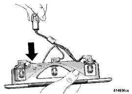
**Removing Connector from Tab**
